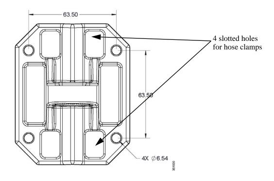
Figure 5 Wall-Mount Bracket and Dimensions (in millimeters)
